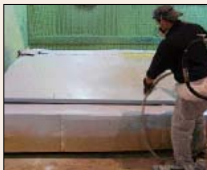
A composite fire barrier for the Boeing 777, coated by FPCL with an epoxy intumescent fire coating.
